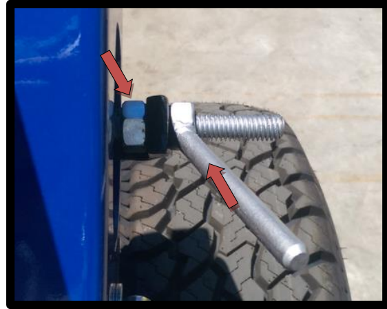
Two nuts which adjust choke
